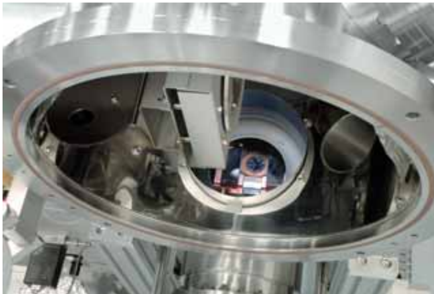
E-beam source well shown in-situ
